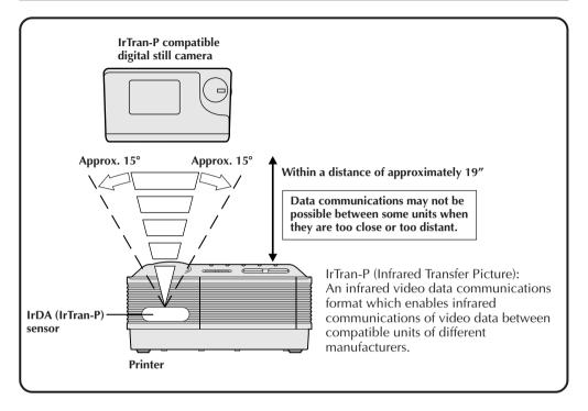
Video data communications with the IrDA (IrTran-P) infrared communications system can be accomplished only between one transmitter and one receiver.
